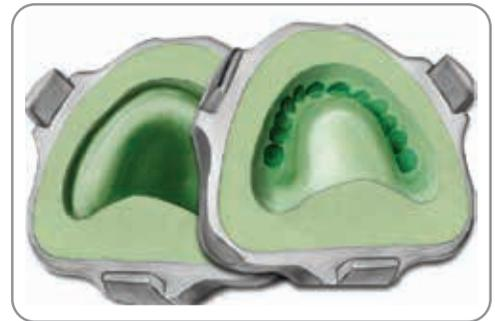
7. Create a mixture of 30% barium sulfate and cold-cure acrylic resin. Pour the mixture into the tooth areas only. Allow the acrylic resin to set per the manufacturer's instructions. Create a mixture of 10% barium sulfate and coldcure acrylic resin. Pour the mixture into the flask. Close the flask tightly. Allow the acrylic resin to set.
